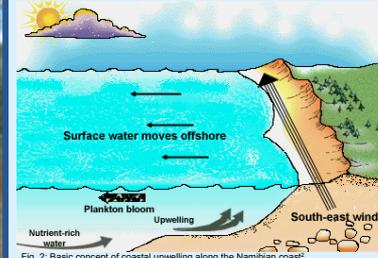
Fig. 2: Basic concept of coastal upwelling along the Namibian coast<sup>2</sup>
