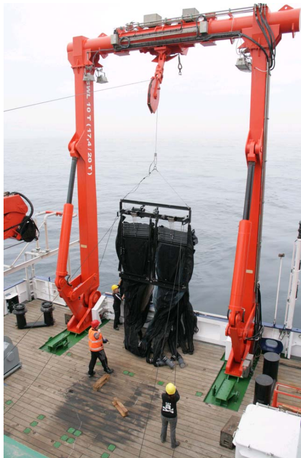
Figure 8: Picture of a 1 m 2 -Double-MOCNESS device with 18 nets (9 left nets, 9 right nets) with a mesh size of 333 µm.
