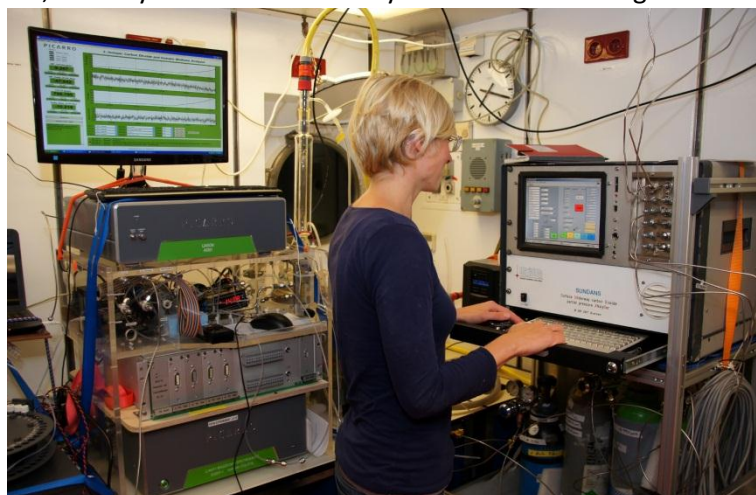
Underway systems continuously measure salinity, temperature, oxygen, pH, CO 2 and CH 4 along the M100/1 cruise track and document the surface expression of a filament cross section
