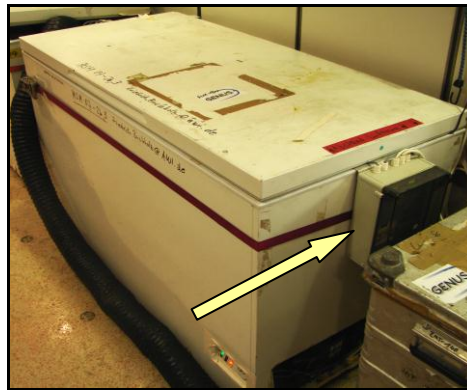
Figure 2: Modified freezer for krill maintenance equipped with temperature regulation device (arrow).
