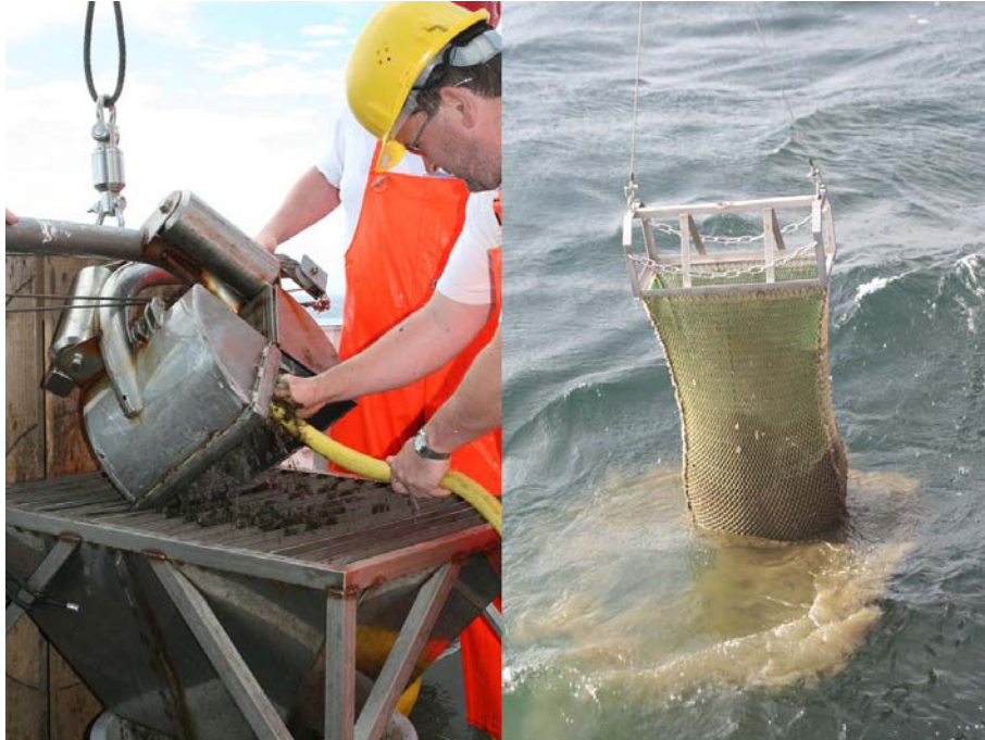
Figure 1.8: The macrozoobenthos was sampled by a 0.1 m 2 van Veen grab (left) and by using a dredge (right).
