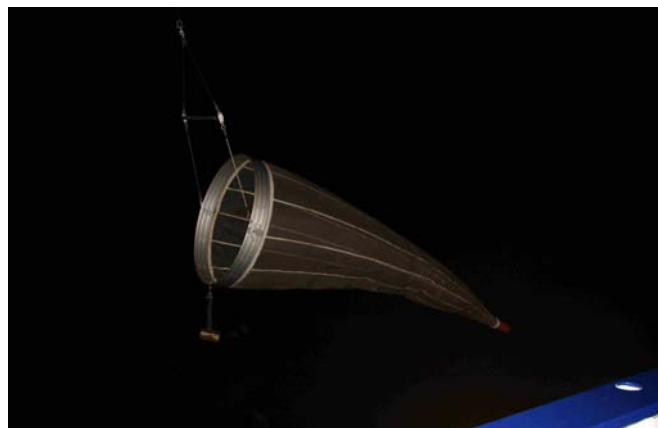
Fig 5.15 Modified Ring Trawl aka Verheye Driftnet
