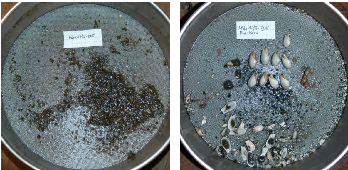
Fig. 5.12 Residuals of the uppermost 7 cm sediment of a single core after sieving through a 500 µm mesh; a) Station 225, 169 m deep, without macrozoobenthos and entirely diffusive solute transport. b) Station 305, 150 m deep, dominated by Nuculana and high bioirrigation
